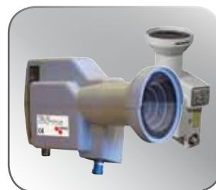
Triax TOL32 optical LNB A high quality, high performance universal LNB, that, in addition to excellent LNB performance, provides a 1310 nm wideband optical output where all four satellite polarities are stacked into one frequency range (950-5450 MHz).
